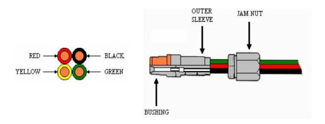
CONSTRUCTION: Jam nut/sleeve - 316 stainless steel, bushing - 4" Viton / 6" Polychloroprene
